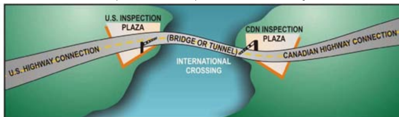
Figure 1.2-1 Components of New or Expanded International Crossing
