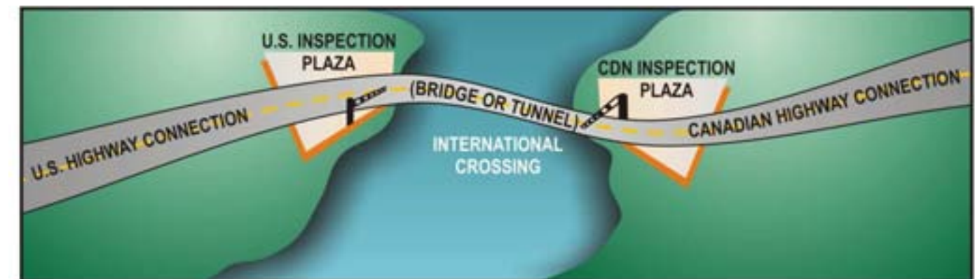
Figure 2.4-1 Components of New or Expanded International Crossing
