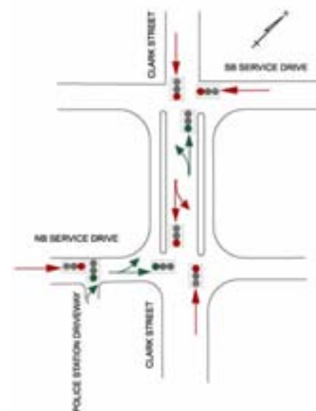
Figure 4.2-18 Clark Street Signalization
